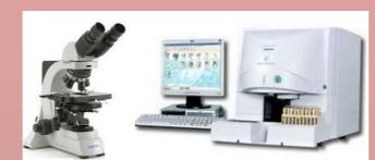
Analyzer: Sysmex 1000i is a fully automated third generation urine sediment flow cytometer. Based on diode laser technology using polymethine dyes specifically staining nucleic acids of urine particles and bacteria. It measures WBC, RBC, bacteria, epithel cells, cast, crystals, yeasts and spermatozoa.
